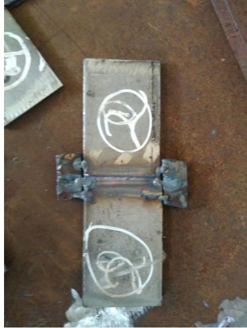
Fig. 3.3 Initial welded specimen
