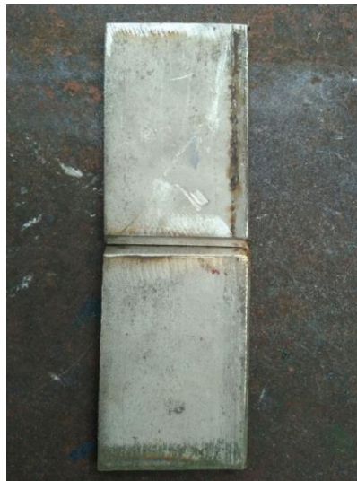
Fig. 3.6 Workpieces readied for Butt welding
