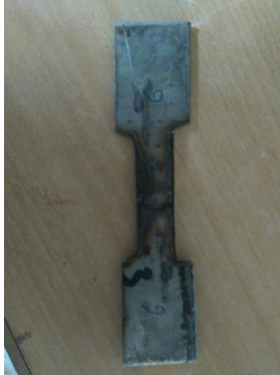
Fig. 3.1 Flat specimen of Stainless Steel SS 202 used for experimentation
