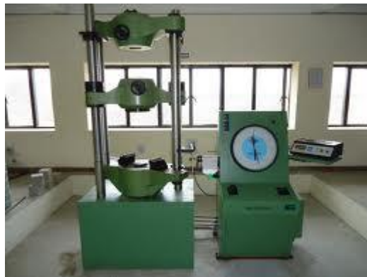
Figure 3.7: Tensile testing machine
