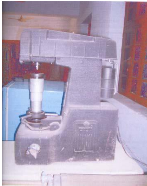
Figure 3.6: Rockwell hardness tester
