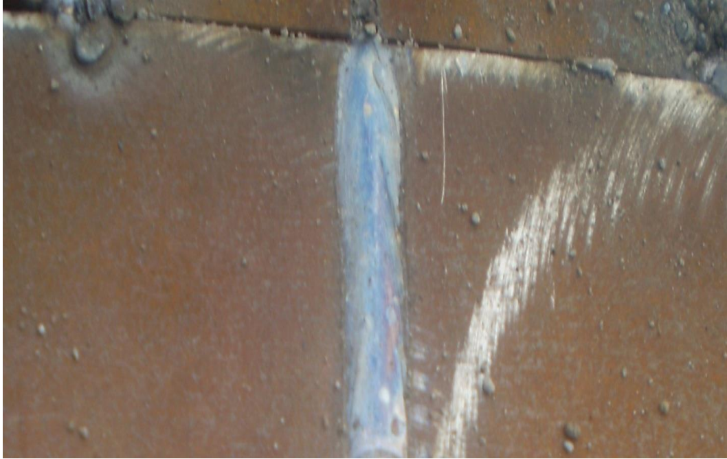
Figure-4.3: Weld obtained at very high speed.
