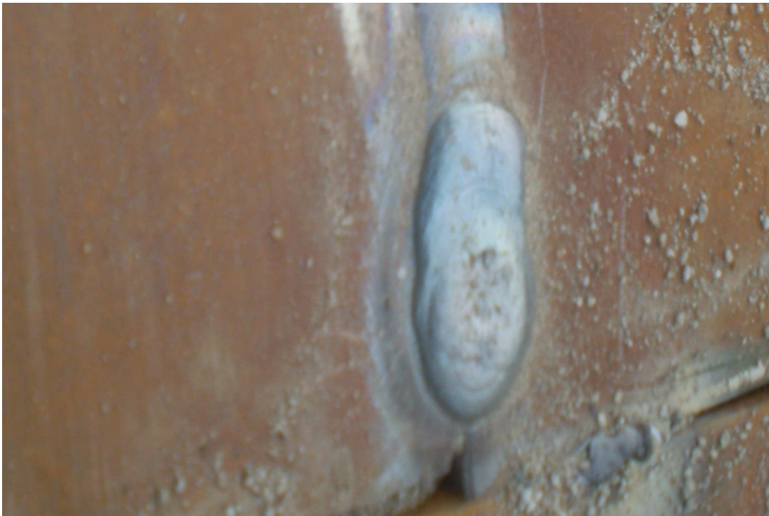
Figure-4.4: Weld obtained at very low speed
