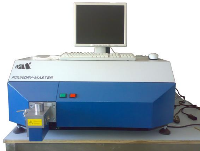
Figure 3.0: Chemical composition tester
