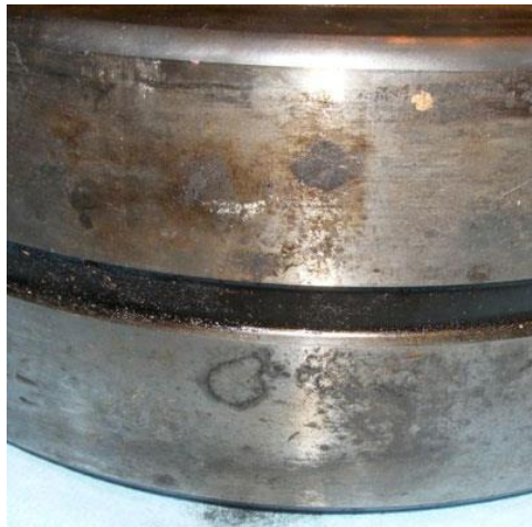
Fretting Marks On Outside Diameter Of Spherical Roller Bearing
