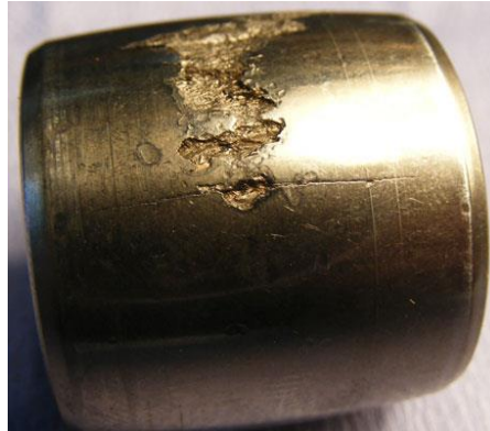
Flaking On The Inner Ring Of Spherical Roller Bearing
