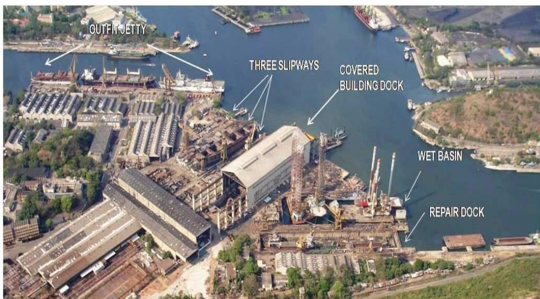
Fig1.1 LAYOUT OF HSL
