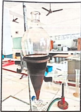
Fig 3.2: Separation of Glycerol and Esters
