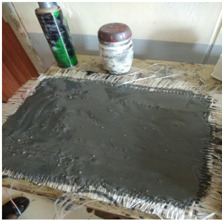
Fig 3.2 Fabrication by hand lay-up method
