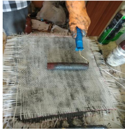
Fig 3.2 Fabrication by hand lay-up method
