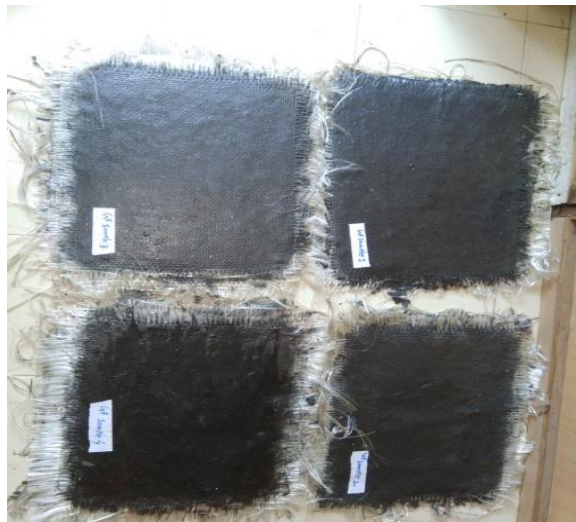
Fig 3.3 Solidified composite sheets after curing 48 hours at room temperature
