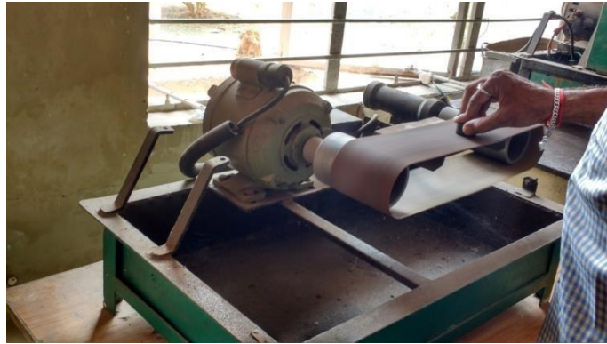
Fig 5.17 Belt grinder for surface finishing operation
