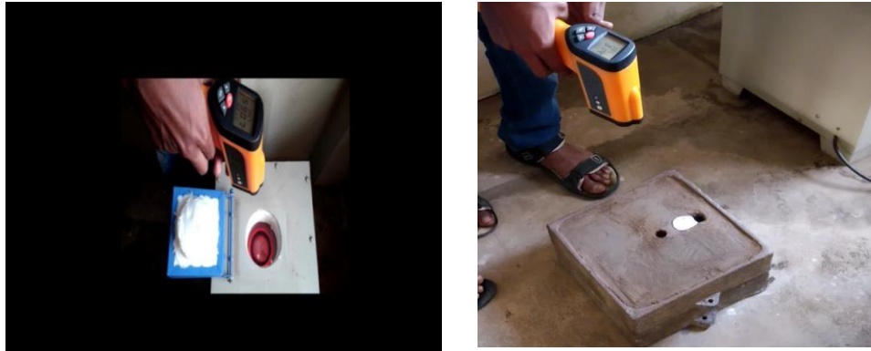
Fig 5.8 and 5.9 Temperature measurement using infrared thermometer
