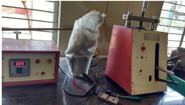
Fig 5.15 Specimen mounting press
