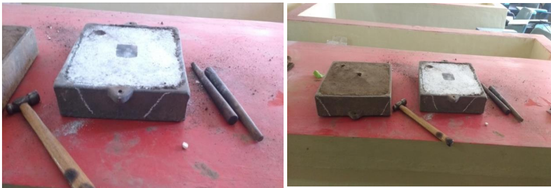
Fig 5.2 and 5.3 Preparation of mold using green sand and single piece pattern
