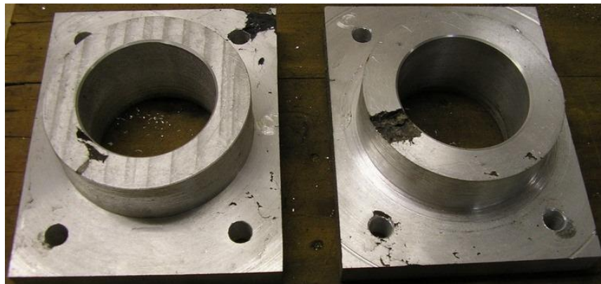
Fig 2.1 Blow holes in casting
