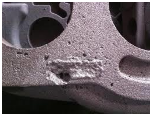
Fig 2.2 Sand inclusion defect
