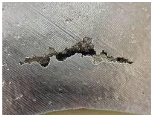
Fig 2.9 Shrinkage defect in casting process
