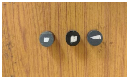
Fig 5.16 Specimens mounted using mounting machine
