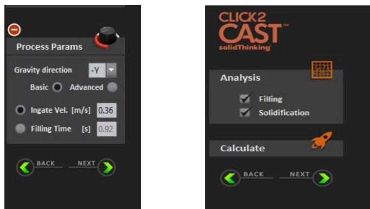
Fig 4.17 & 4.18 Defining process parameters and run calculations
