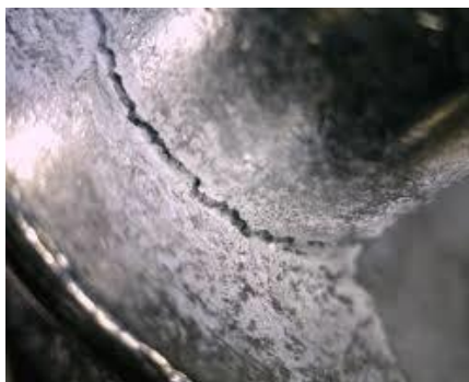
Fig 2.8 Cracks or tears formed during casting
