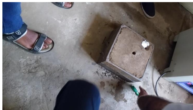
Fig 5.10 Cooling of mold after pouring the molten metal
