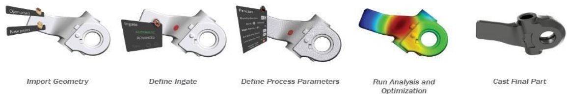
Fig 4.2 Steps in simulation by click2cast software
