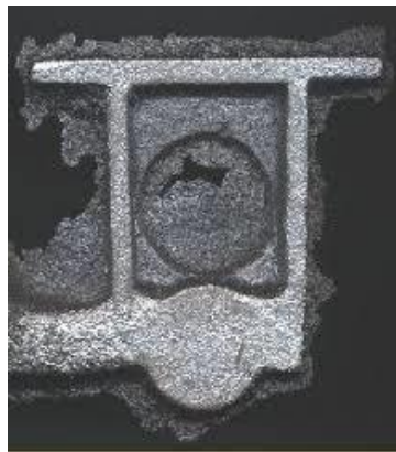
Fig 2.7 Flash defect in casting
