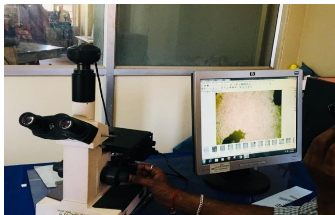
Fig 5.18 Observation of micro structures using inverted trinocular microscope
