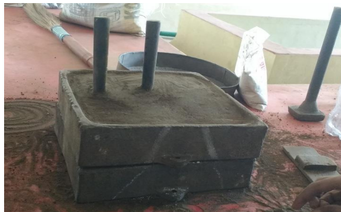
Fig 5.4 Prepared mold with gating system
