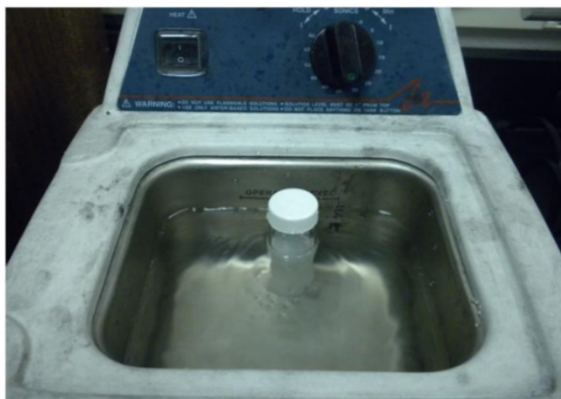
Fig: 3.2 Branson 1510 Ultrasonic Cleaner Ultrasonic ting an Alumina Nanofluid.
