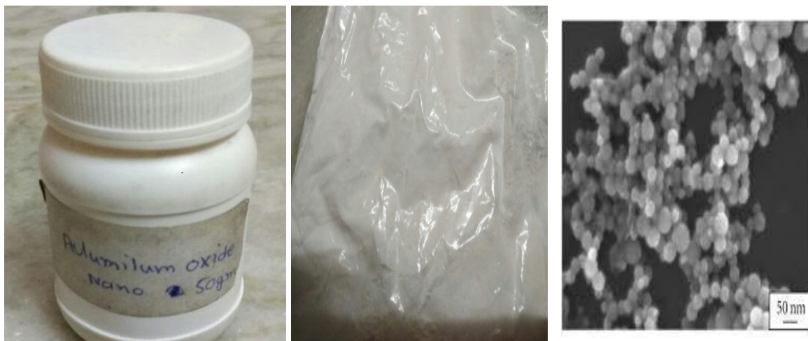
Fig: 3.1 (a) Alumina oxide (50nm) Fig: 3.1 (b) Aluminium powder Fig: 3.1 (c) \text{Al}_2\text{O}_3 structure
