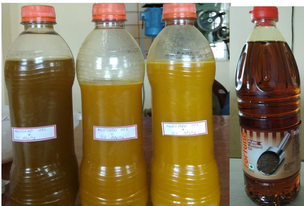
Figure 3.11 Prepared samples with 0%, 1% , 2%, 3% \text{Al}_2\text{O}_3 in Mustard oil
