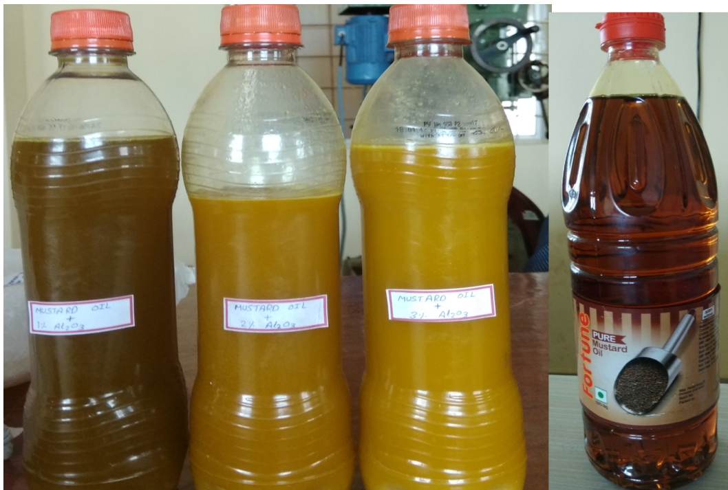
Figure 4.2 Prepared samples with 0%, 1% , 2%, 3% Al 2 O 3 in Mustard oil
