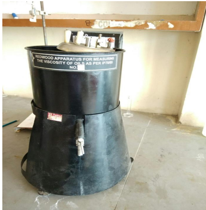
Figure: 3.9 Redwood Apparatus For Measuring the Viscosity of oil
