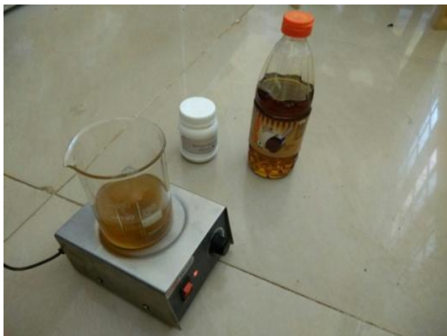
Fig: 3.4 Amalgamation of Mustard (99 %) and 1% Al 2 O 3 Sample preparation through stirring process
