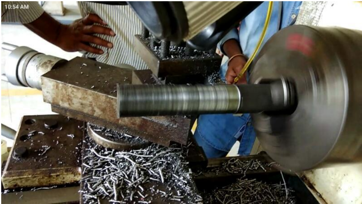
Fig: 4.9 Machining with pure mustard oil
