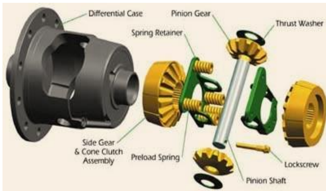
Fig 1.9 Cone Clutch LSD
