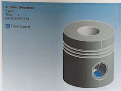
FIG 4.1 Fixed Support at Piston Pin
