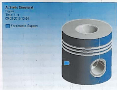
Fig 4.2 Frictionless Support to Sidewalls
