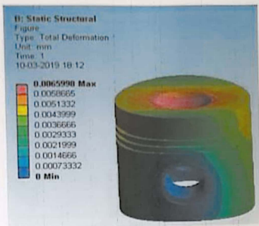
FIG 5.12-Total deformation of hemi-spherical crown for Al 2618.
