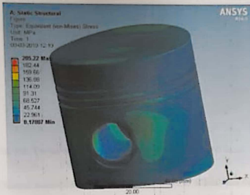
FIG 5.4- Variation of Equivalent stress for a piston with flat crown for Al 6061.
