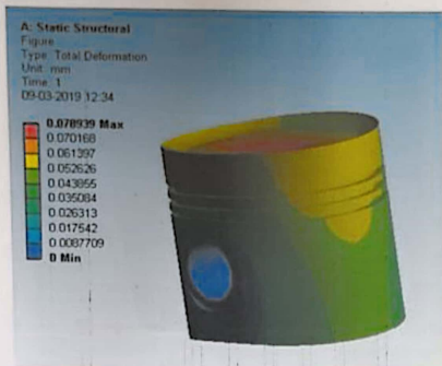
FIG 5.2-Total deformation of dished crown for Al 6061.
