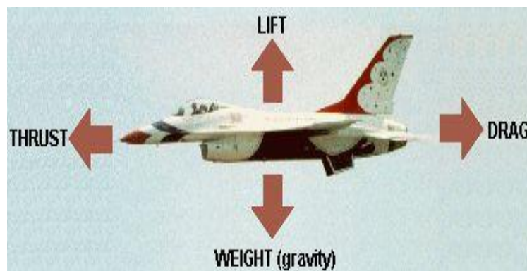
Fig.1.9 Lift and Drag Forces on Aircraft.
