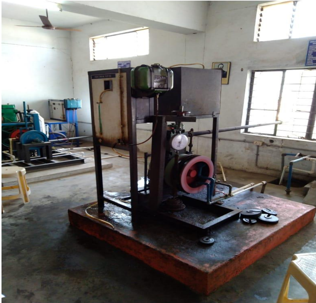
Fig 4.2: Four Stroke, Single Cylinder, Vertical Diesel Engine
