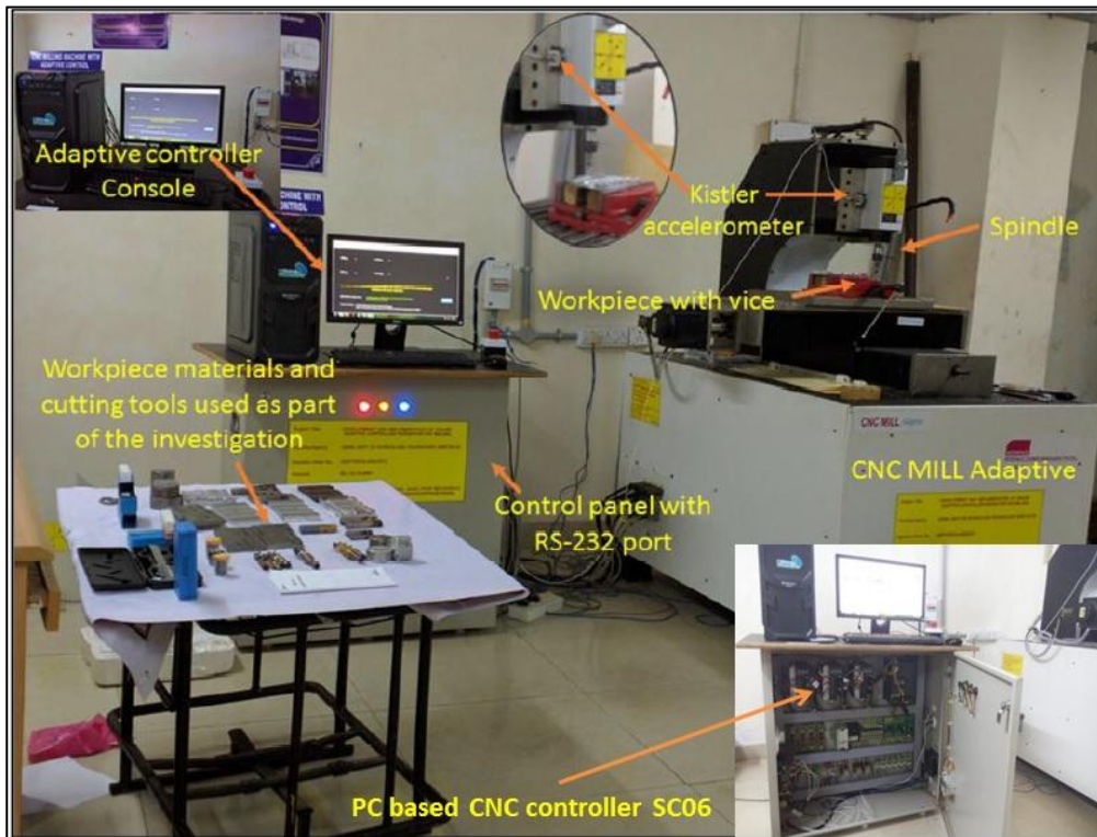
Figure 1 Investigational test setup with workpieces and cutting tools
