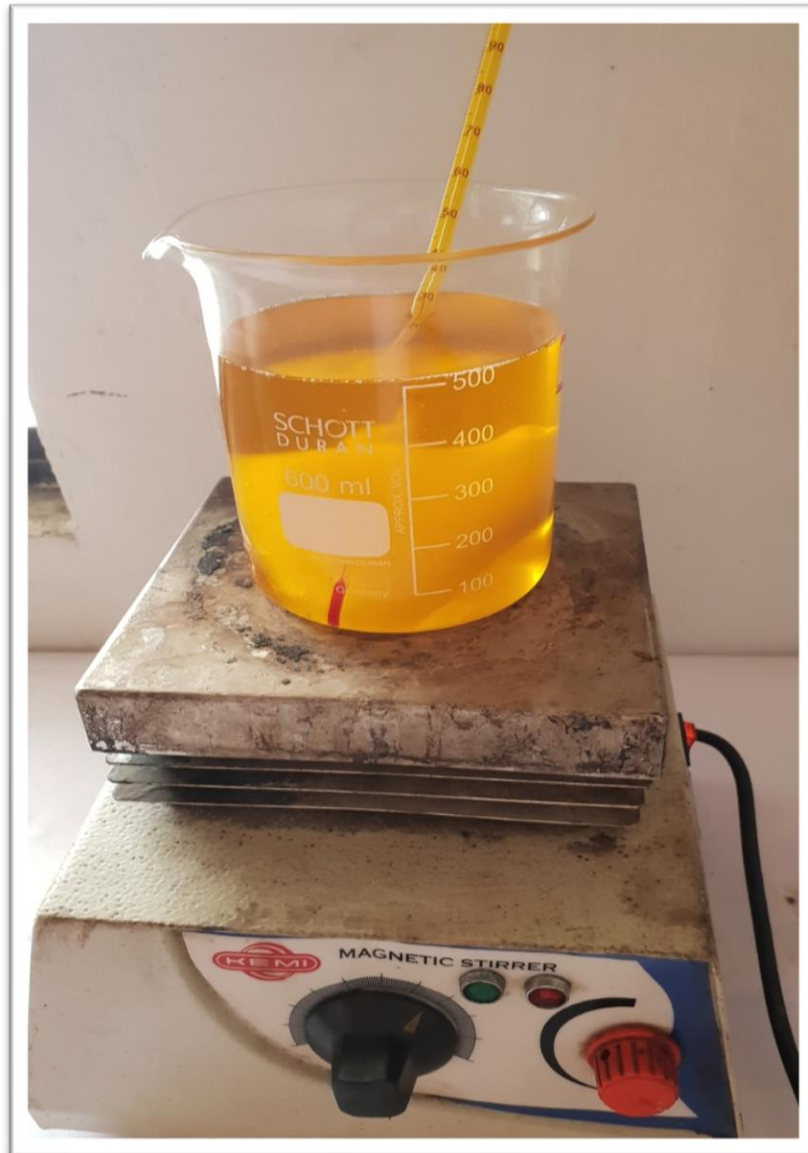
Fig 3.4.1 HEATING OF OIL
