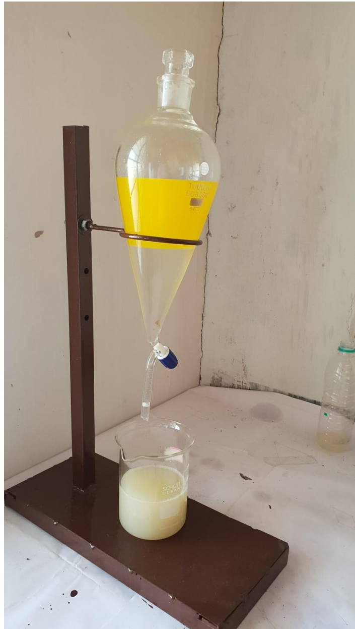
Fig 3.4.4 REMOVAL OF EXCESS SOAP
