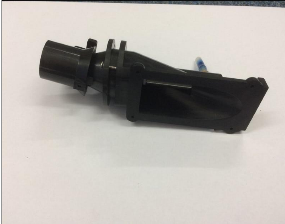
Fig.3.15 3D Printed Water Jet Propulsion System
