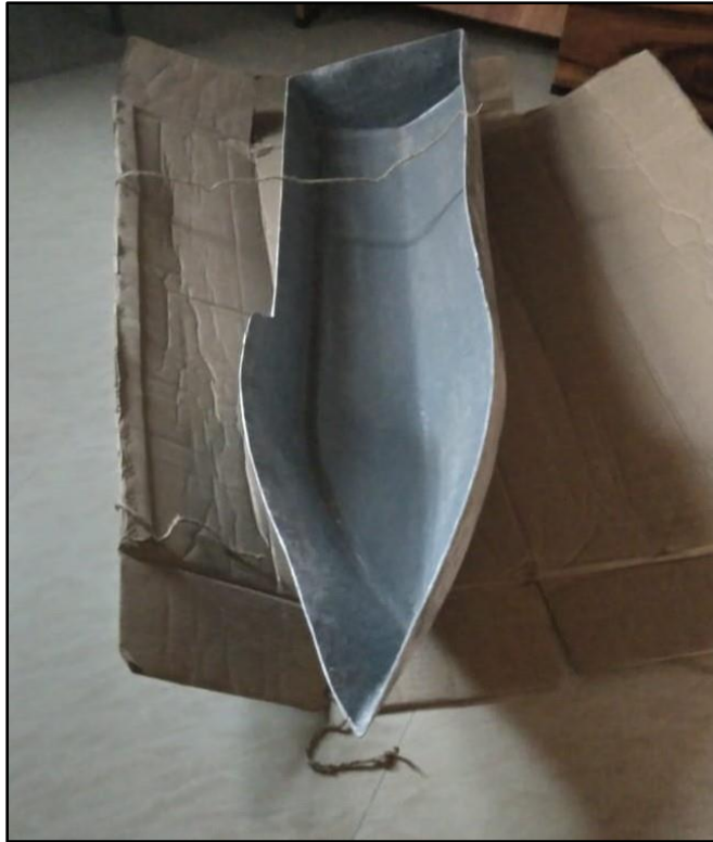
Fig.3.7 Bare hull of fiberglass
