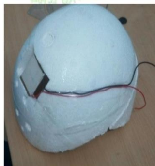
Fig 4.2 Attachment of peltier module in grooves
