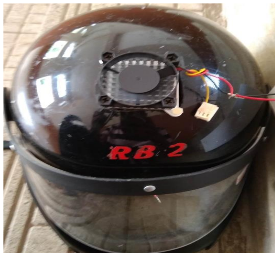
Fig 5.6 Assemble of thermoelectric module and heat sink
