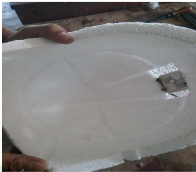
Fig 5.2 Making of Groove in inner shell
