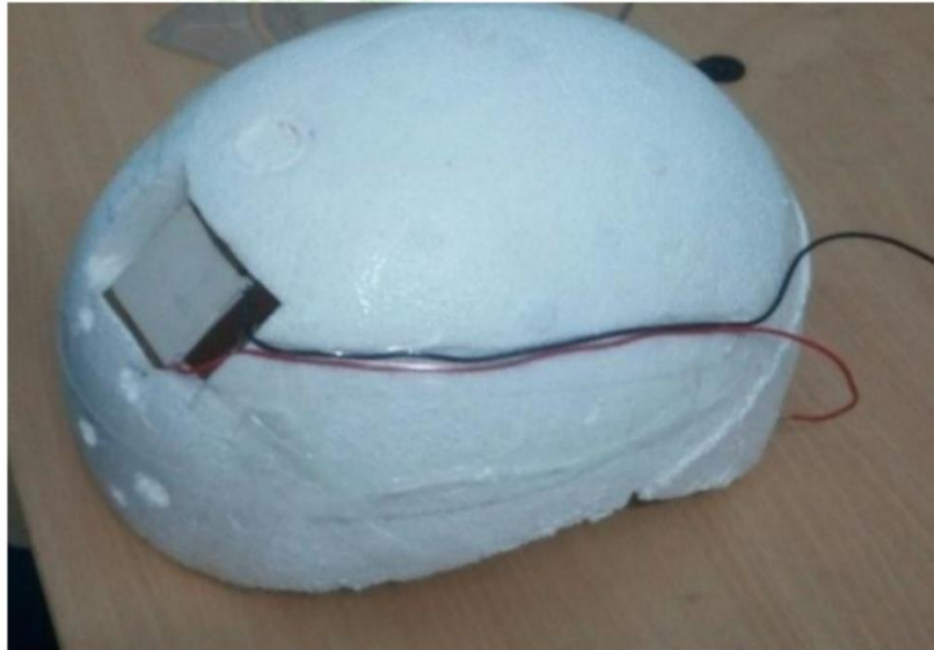
Fig 5.3 Installing Thermoelectric Module in grooves
