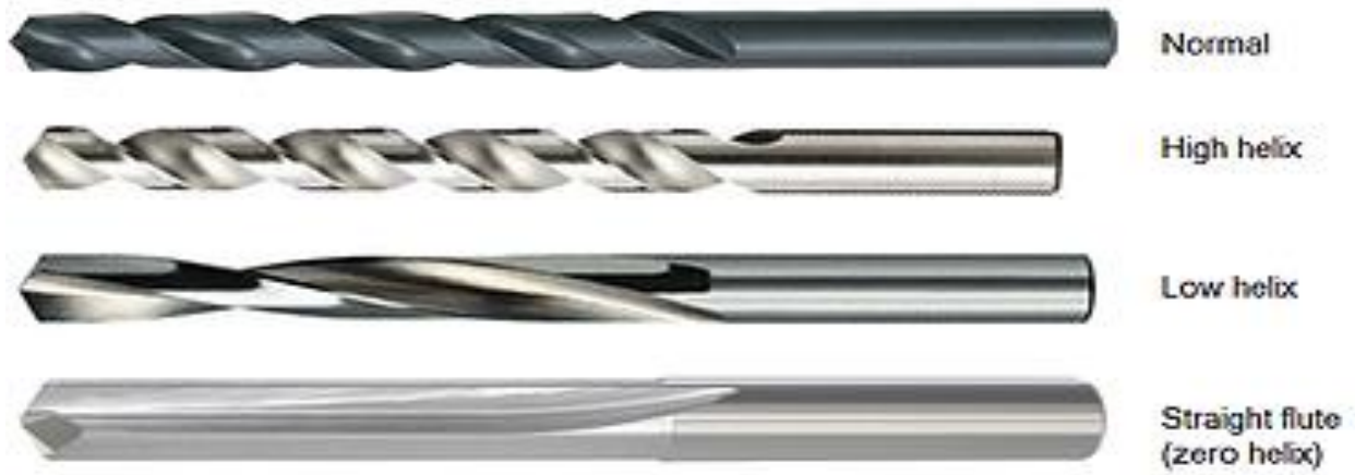
Figure 1.5 Drills Based on Helix Angle
