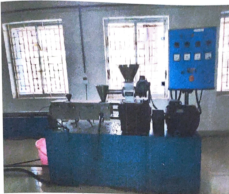
Figure 3.4: Twin Screw Extruder fitted with circular die powered by servo motors operated at 175°C with a rotor speed of 100 rpm for 5 minutes.
