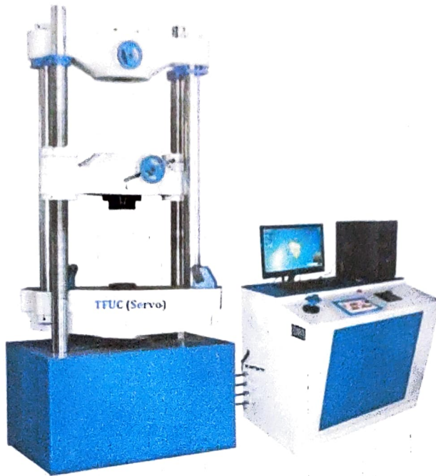
Figure 6.1: Universal testing machine (UTM) for performing tensile test on the specimen
