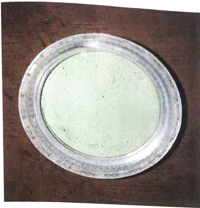
Figure3.3: Tungsten disulphide Nano powder (WS2) supplied in airtight plastic container
