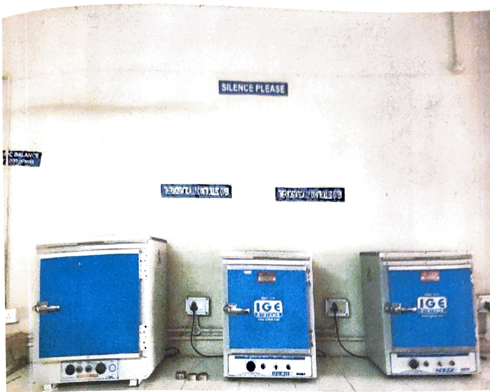
Figure 3.2: Thermostatically controlled ovens used to preheat acetyl copolymer at its softening temperature of 80°C for about 24 hours
