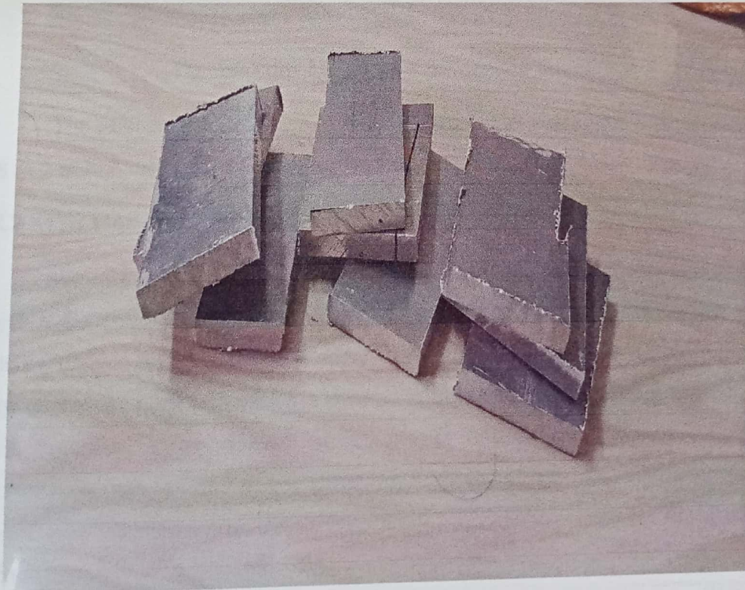
Fig. 3.5 Billets of Al6061 material
