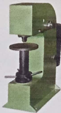
Fig. 3.13 Brinell Hardness test
