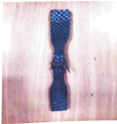
FIG-4.3.2 Tensile test specimen after failure
