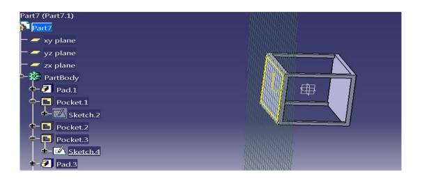
STEP-4:SKETCH A CIRCLE ON THE TOP OF THE FRAME AT REUIREDPOSTION TO OBTAIN THE PULLEY AND SHAFT
