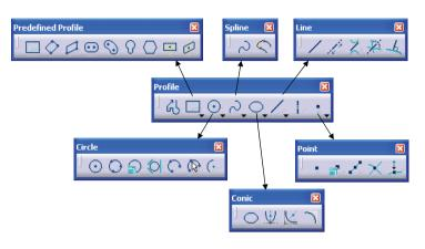
toolbar contains many sub-toolbars. Most of these sub- toolbars contain different options for creating the same geometry. For example, you can create a simple line, a line defined by two tangent points, or a line that is perpendicular to a surface. Reading from left to right, the Profile toolbar contain the following commands.
