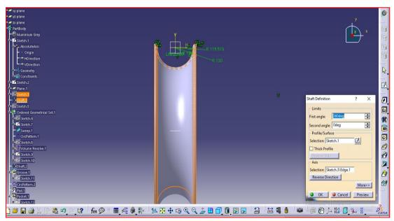
STEP-3: DRAW THE PROFILE OF TYRE USING SPLINE AND CIRCLE COMMAND FROM PROFILE TOOL BAR AS SHOWN IN FIGURE
