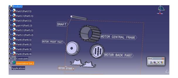
STEP-2: USE COINCIDE COMMAND TO COINCIDE THE AXIS OF MOTOR FRONT, BACK AND CENTRAL PART.
