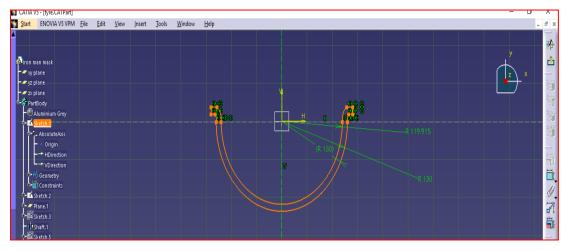
STEP-2: BY USING SHAFT COMMAND WE HAVE EXTRUDED THE ABOVE PROFILE 360<sup>0</sup> MENTIONED IN THE STEP-1 AS SHOWN IN THEFIGURE
