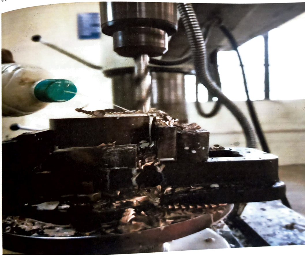
Fig 4.3 : drilling of work piece
