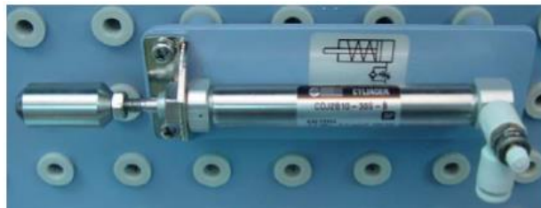
Fig 1.3 b) Single acting cylinder
