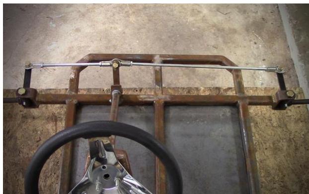
Fig 1.2- Steering Mechanism of a Go-Kart
