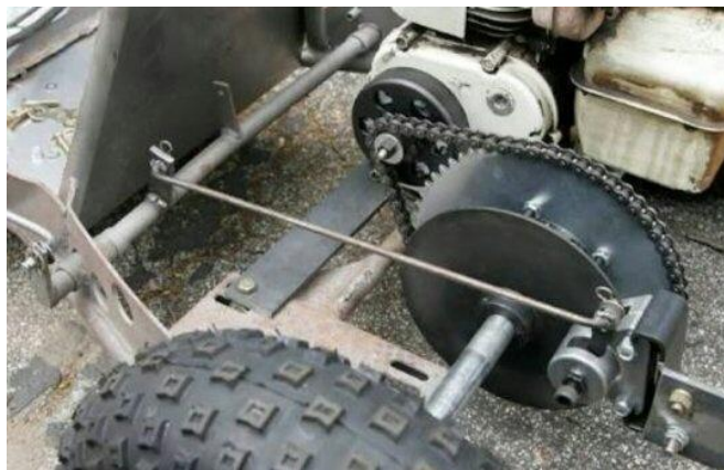
Fig 1.3- Transmission of a Go-Kart
