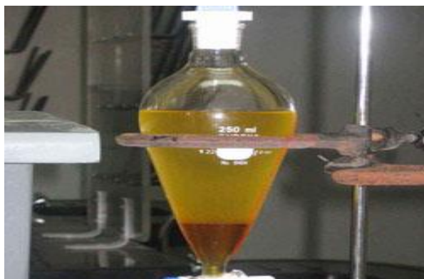
Fig3.6 transesterification of coconut oil
