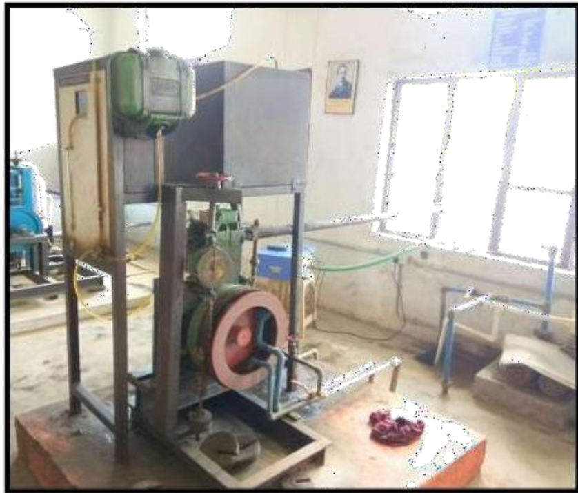
Fig : 4.1 Four Stroke Vertical Diesel Engine With Brake drum Setup
