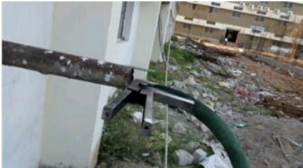
Fig:4.4 Exhaust Pipe clamped to analyser
