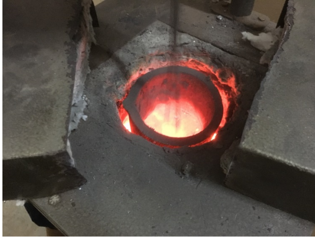
Fig 1.3 Close view of Stir casting process
