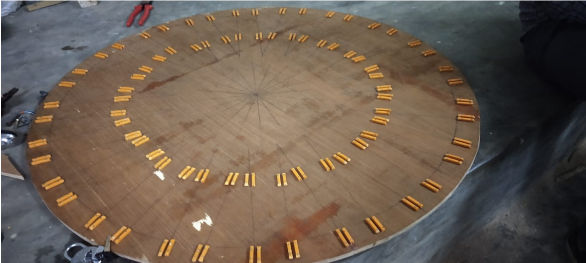
Fig.5.2 Grooves at base and lid plate
