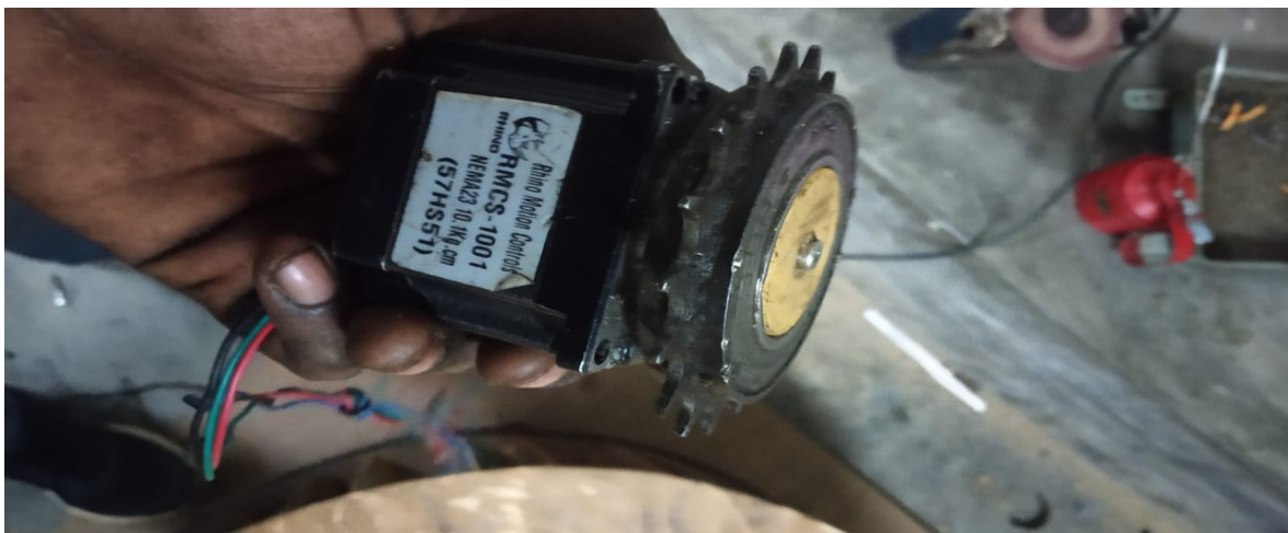
Fig.5.6 Stepper motor with sprocket
