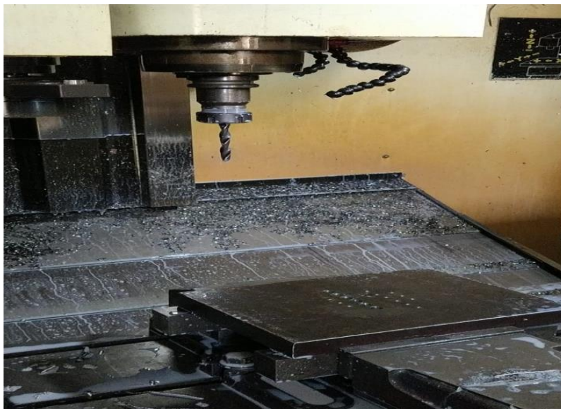
Fig. Drilling Operation
