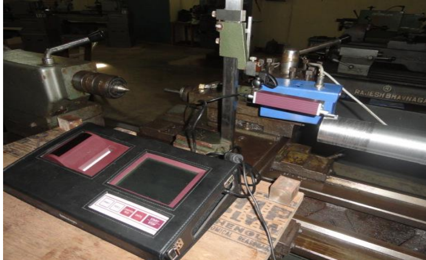
Figure 4. 1: Surface Roughness Testing Apparatus
