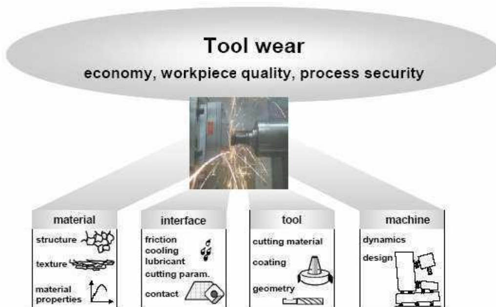
Fig.1.6. Influencing elements of tool wear
