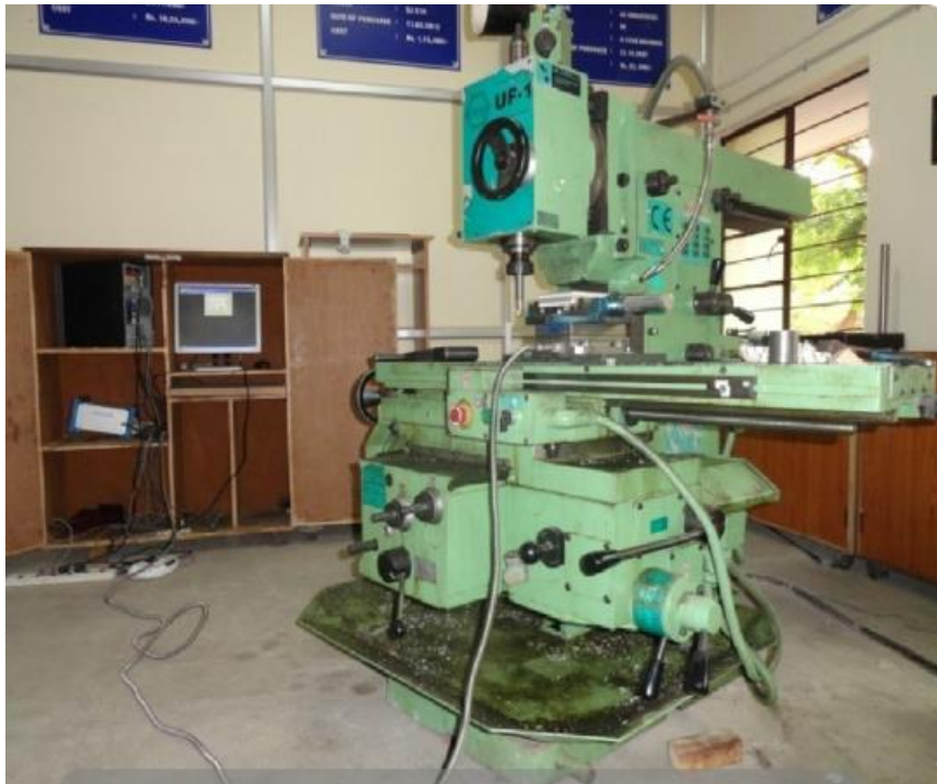
Fig.3.1. End milling operations were carried out in a BHARAT FRITZ WERNER BF-1 universal milling machine with 2.2 kW motor capacity.
