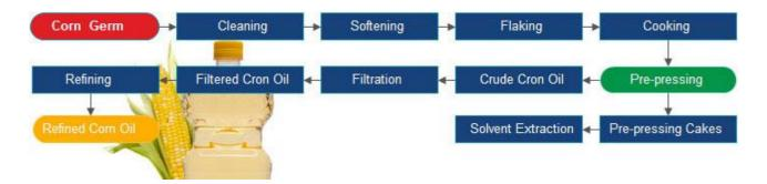
Generally, corn oil is produced by expeller pressed method, then solvent-extracted the oil cake by using hexane or iso hexane. The solvent is then recovered for re-use by evaporation. The extracted crude corn oil is then sent to refining plant (including degumming, dewaxing, alkali treatment) to get high quality edible corn germ oils.
