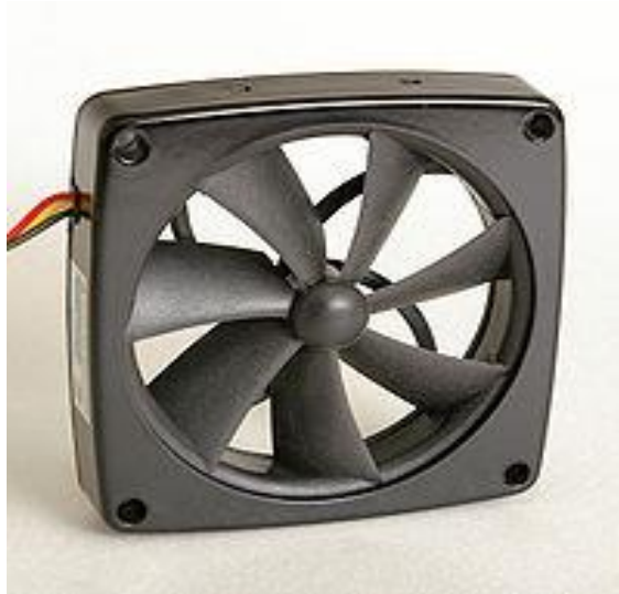
Fig 4.9: Axial flow cooling fans
