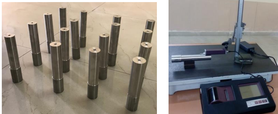
Figure 4.1. AISI 316L workpiece after machining and surface roughness tester SJ-301
