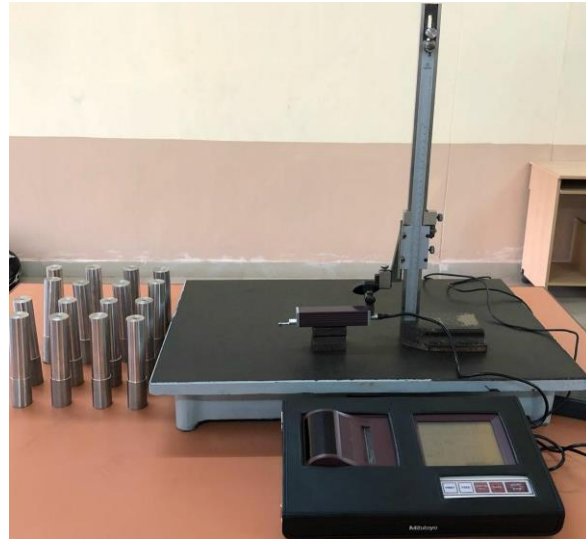
Figure 4.5. AISI 316L workpiece after machining with surface roughness tester SJ-301
