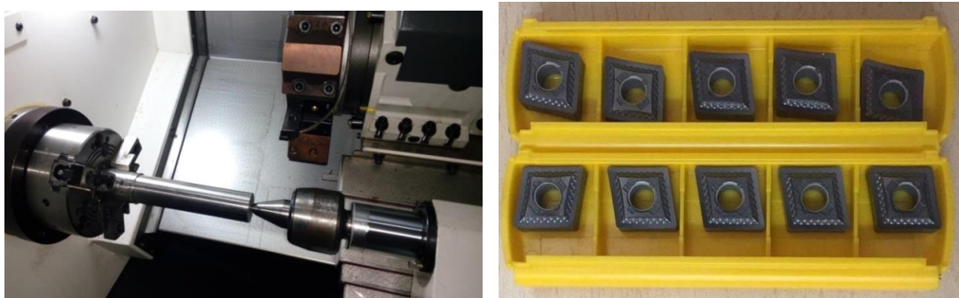
Figure 4.2. CNC lathe with Fanuc-0i control system and coated carbide inserts.
