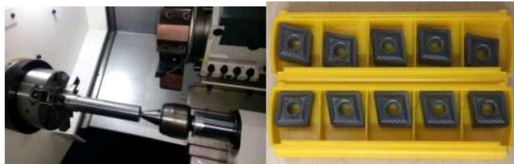
Fig.5 CNC lathe with Fanuc-0i control system and coated carbide inserts
