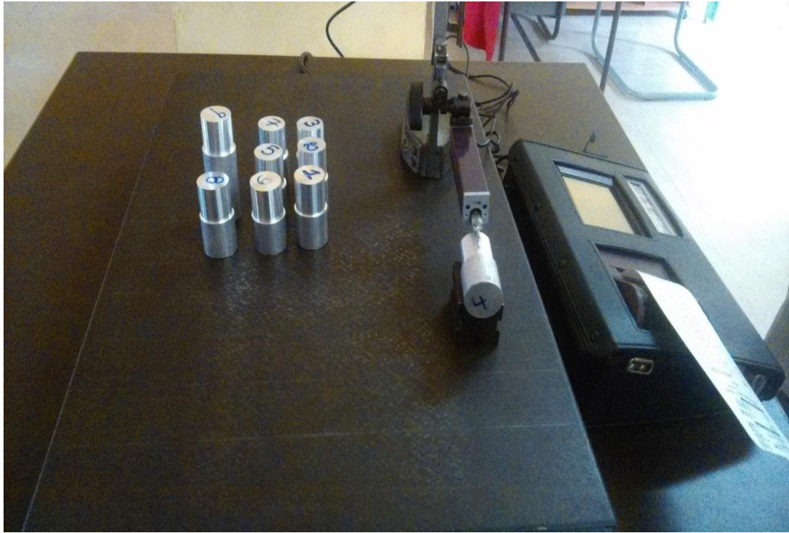
Figure 4.6. Surface Roughness Measurement Set-up
