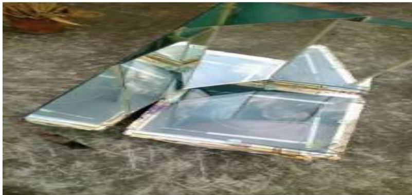
Fig 4.10-5 segment parabolic solar cooker
