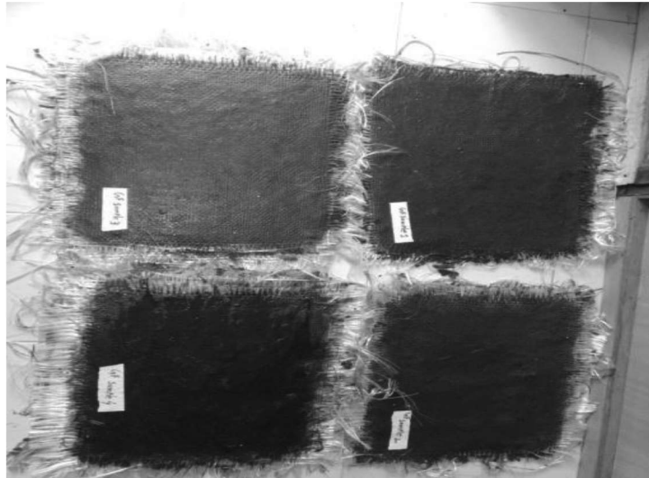
Fig 3.3 Solidified composite sheets after curing 48 hours at room temperature
