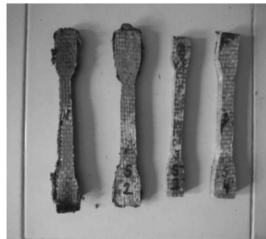
Fig 4.2(b) Specimens after testing
