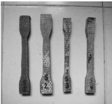
Fig 4.2(a) Specimens before testing
