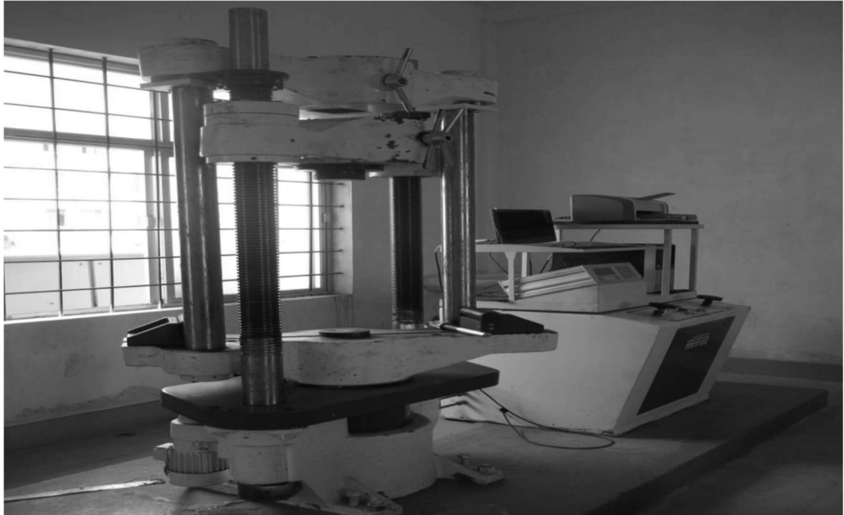
Fig 4.1 Tensile Testing Machine
