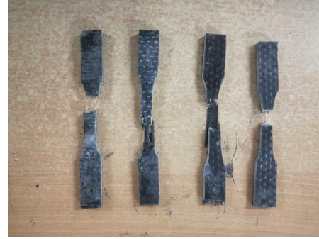
Fig-4.3.2 Tensile test specimen after failure
