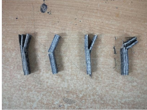
Fig - 6.2.2 Impact test specimens after failure
