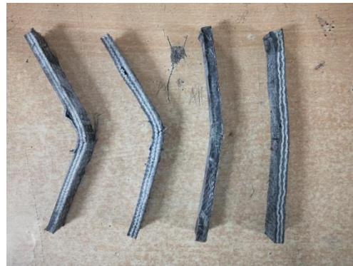
FIG-5.3.2 Specimen after performing Flexural Test
