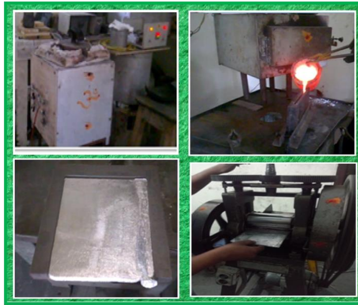
Figure 4.1 (a-d) shows the Electrical Resistance Furnace (b)Pouring molten mixture into the preheated permanent mold (c)Al-Mg-Mn-Sc-Zr as cast plate (d) Cold rolling of plate
