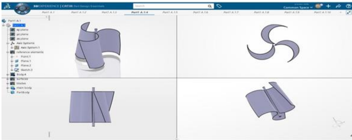
Fig 4.2.3 Savonius Wind Turbine with 30 deg twist in blades
