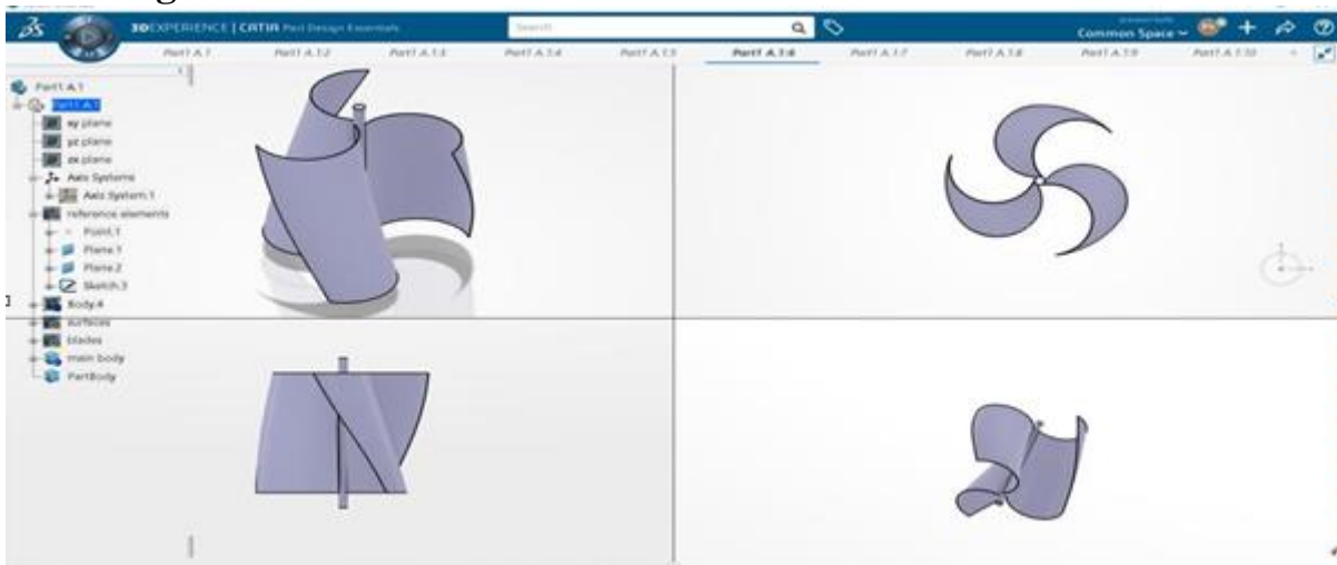
Fig 4.2.5 Savonius Wind Turbine with 50 deg twist in blades
