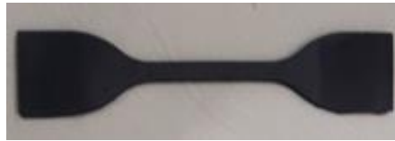
Fig. 4.6 Tensile testing rubber specimen
