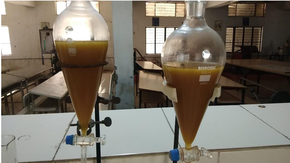
Fig 3.2: Separation of Glycerol and Esters
