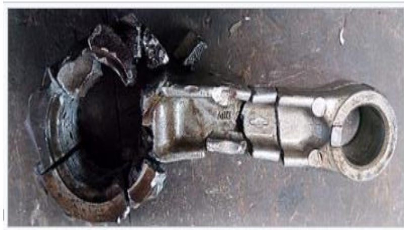
Fig 1.5: Connecting rod that initially failed through fatigue, then further damaged from impact with crankshaft
