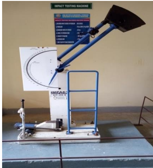
Fig 4.10 Impact test equipment and impact test specimen
