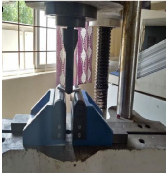
Fig 4.9 UTM and Bending test specimen
