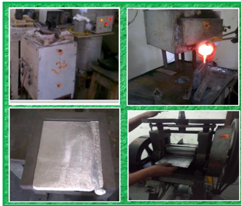
(a) Electrical Resistance Furnace (b) Pouring molten mixture into the preheated permanent mould (c) Al-Mg-Mn-Sc-Zr as cast plate (d) Cold rolling of plate Fig..4.1 Fabrication process of Al-Mg-Mn alloy
