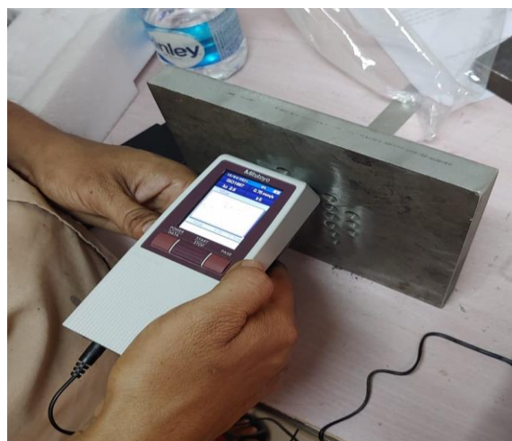
Fig 4.8 Surface Roughness Tester measuring
