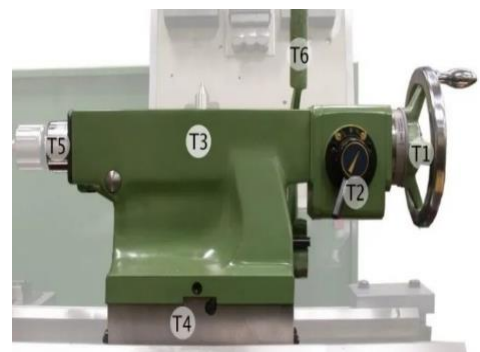
Figure 1. 5: Tail Stock of a Lathe Machine
