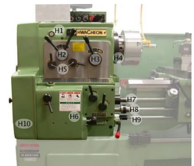
Figure 1. 4: Head Stock of a Lathe Machine
