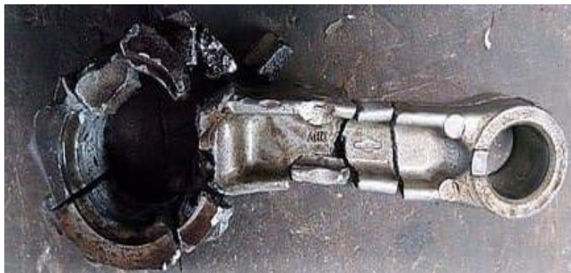
Fig 1.4: Connecting rod that initially failed through fatigue, the further damaged from impact with crankshaft
