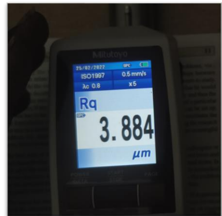
Fig 4.10 Tester displaying Rq value
