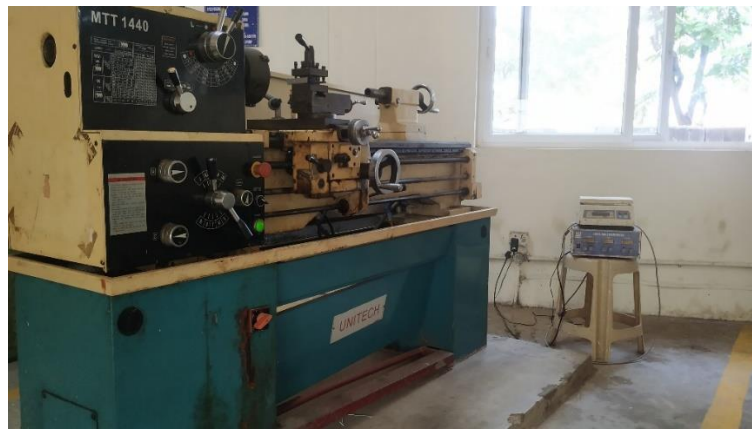
Fig. 4.1 Centre Lathe with digital weighing machine
