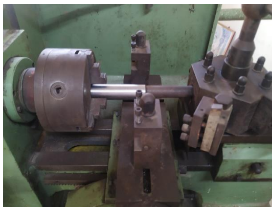
Fig. 4.2 Workpiece in position for center drilling
