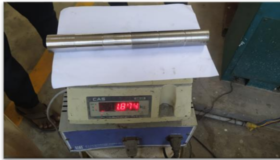
Fig. 4.5 Checking workpiece weight after machining
