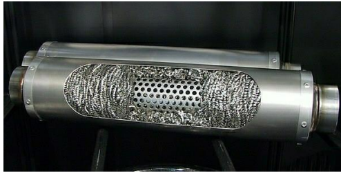
Figure 1.17 Combined Type Muffler
