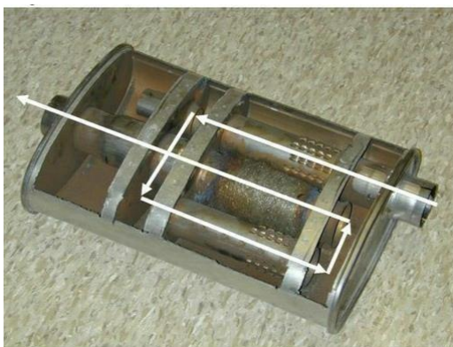
Figure 1.14 Wave Cancellation Type Muffler
