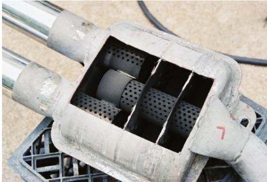
Figure 1.13 Baffle type Muffler
