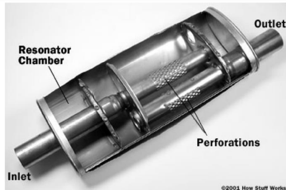
Figure 1.8 Straight Through Absorption Muffler
