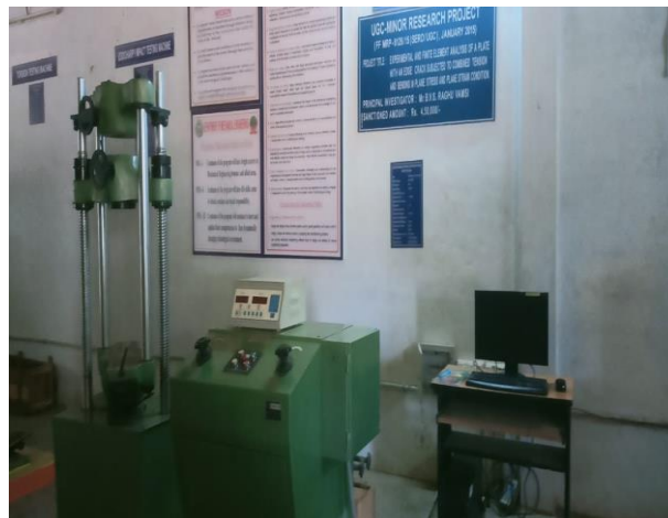
Figure 4.7: Universal test machine (UTM)
