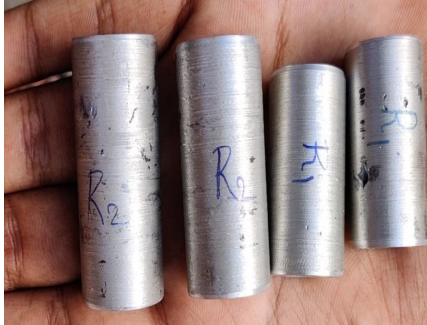
Figure 4.11: Compression pieces after machining
