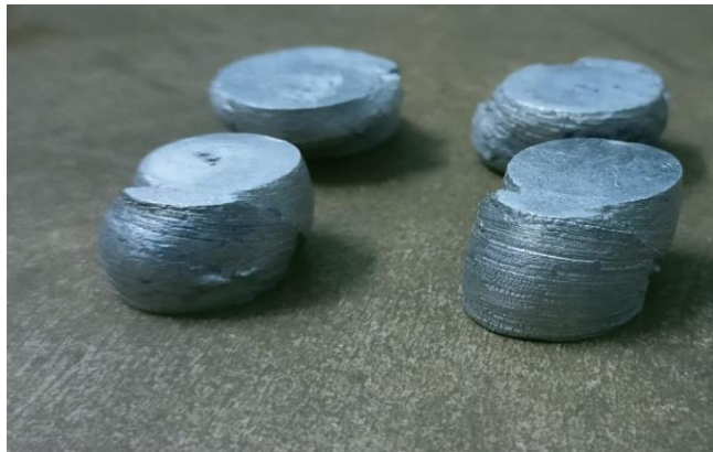
Figure 4.12: Compression pieces after testing
