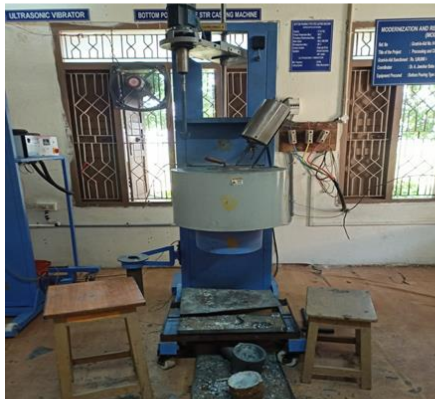
Figure 3.7: Stir Casting Furnace
