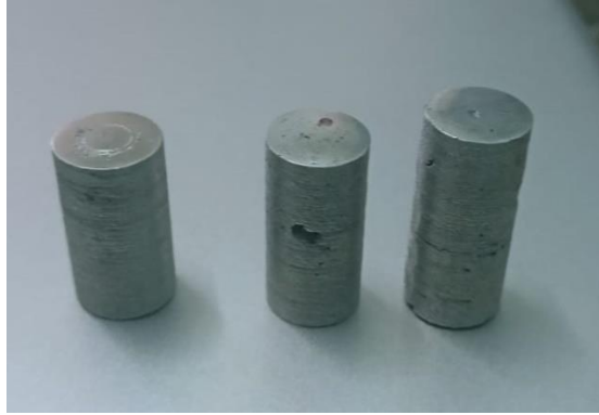
Figure 4.15: Hardness test specimen after testing
