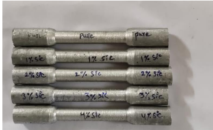
Figure 4.6: Tensile pieces after machining
