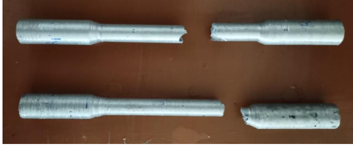
Figure 4.9: Tensile test specimen after testing
